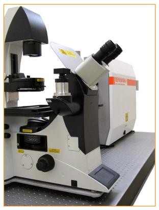
inVia equipped with both inverted and upright microscopes.
