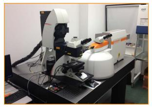
Combined Raman and confocal laser scanning microscope
